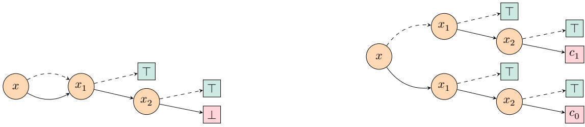
(a) A decision-DNNF circuit produced by a top-down solver with syntactic caching.
